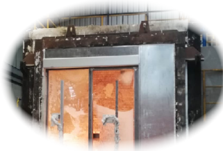
Fire proof glazed sliding door EW60 rating
